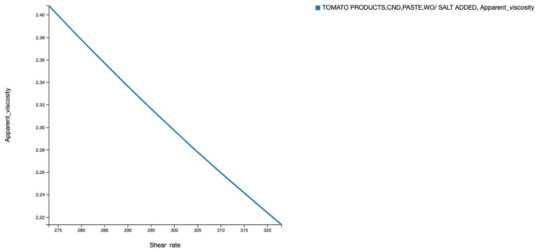
The apparent viscosity of tomato paste decrease with increasing shear rate due to the shear-thinning behavior of the material, where the alignment of suspended particles and breakdown of structure reduce the resistance to flow. This allows the tomato paste to become less viscous under high shear conditions, making it easier to handle and process.
