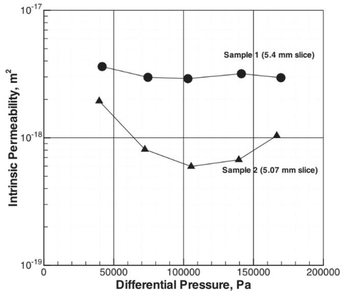
Figure 5 Water permeability in raw potato tissue of a different thickness.
