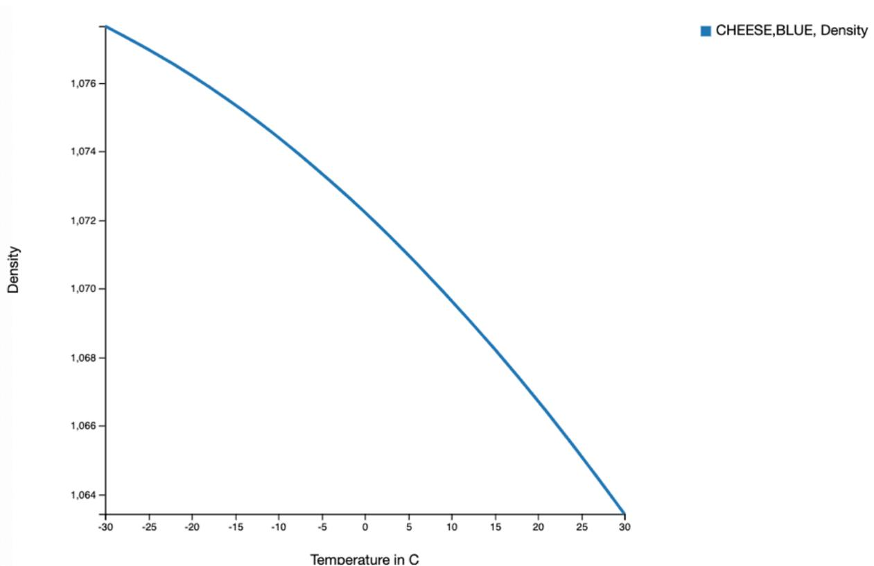
The density of blue cheese decreases with increasing temperature because heat will cause the fat and water content to expand and increase the volume while the mass remains constant. The molecules will move farther apart, and the cheese structure will become less compact as thermal expansion leads to lower density.
