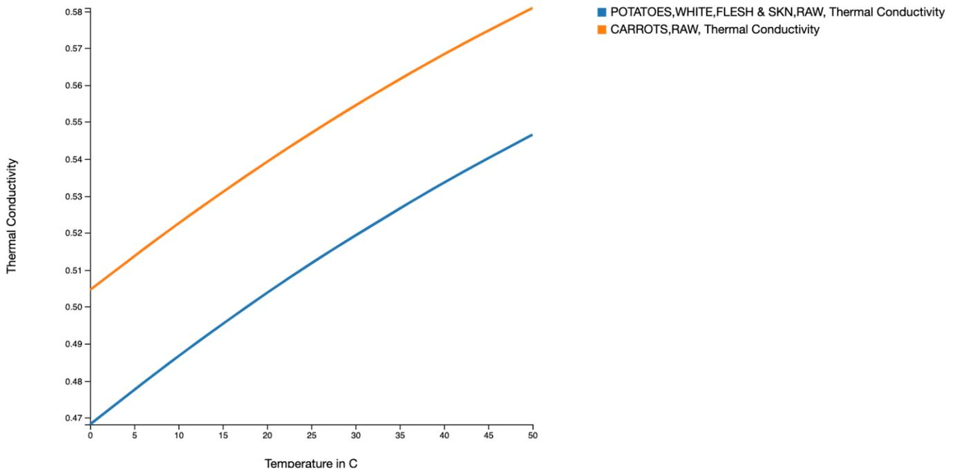
The graphs of thermal conductivity of these two materials is different despite using the same formula because of the material composition, shown below. White Potatoes (left) and Raw Carrots (right).
