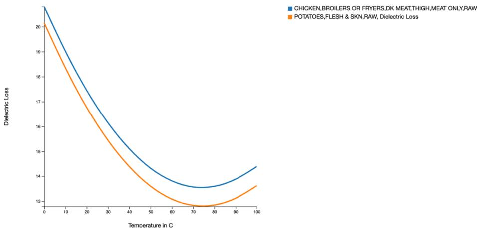
The dielectric loss of raw chicken and potatoes decrease from 0 to 75 °C due to reduced molecular relaxation and loss of water content but curves up after 75 °C because proteins and starches denature at this temperature. The dielectric loss of chicken is greater than potatoes overall because chicken has higher protein content and less carbohydrate content, both of which contribute to significant dielectric loss, though both materials follow the same trend.
